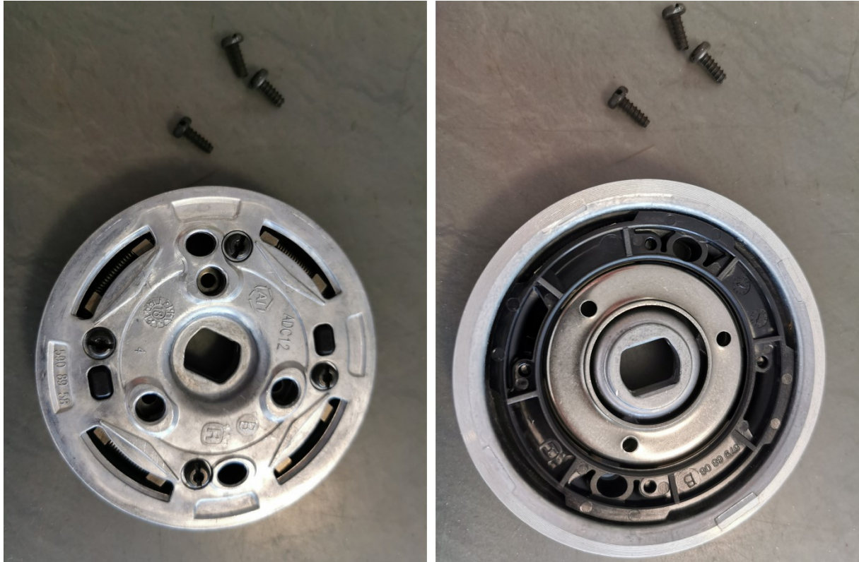
Belt pulley, with disc brake (5) mounted, front and rear side
