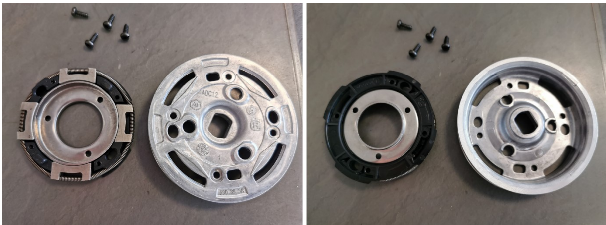
Belt pulley (7) and disc brake (8) dismantled, front and rear side
